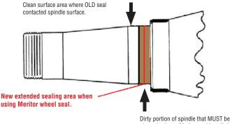
cleaned prior to Meritor seal installation.
